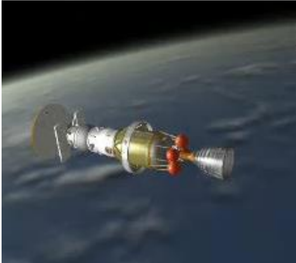
The second stage of Delta II with Mars Polar Lander (03.01.1999)
