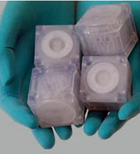
Microsatellite with four control moment gyroscopes
