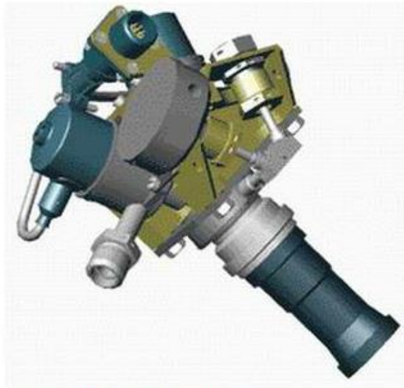
Cyclone-3 LV thruster of 30 N thrust
