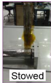
L'Garde Patented Sub-Tg Conical Deployable Booms
