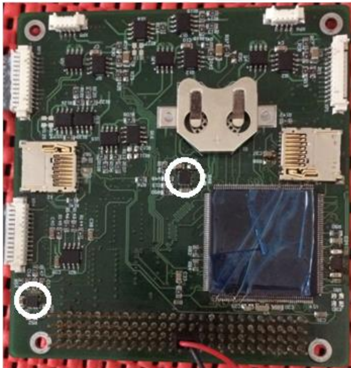
Location of MPU-9250 sensors on OBC of SamSat platform
