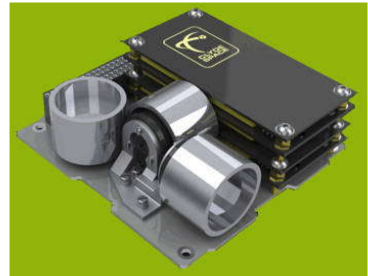
Three-axis attitude control system © Clyde Space
