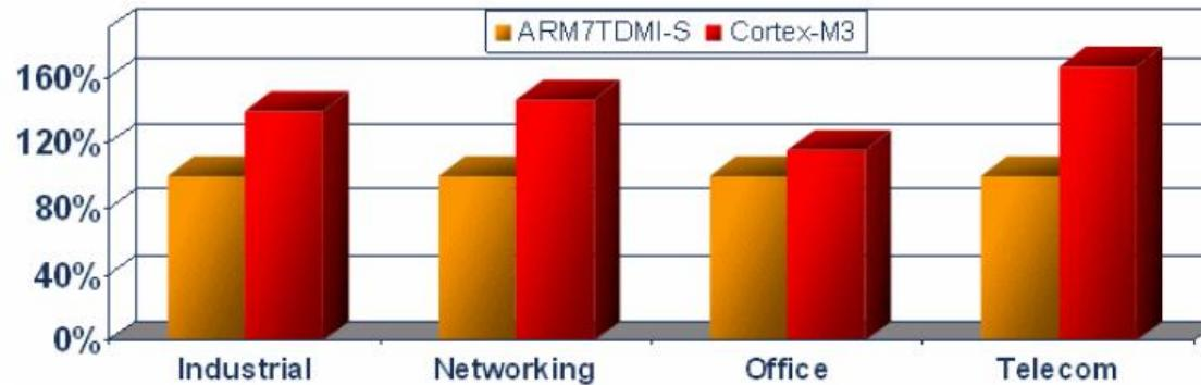
Relative code size for ARM7TDMI-S (ARM) and Cortex-M3 (Thumb-2)
